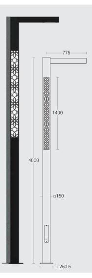
Base plate 250.5 x 14.5thk. 2 Nos. of M16 Nut 2 Nos. of Plain 8 Spring washer 4 Elongated holes 38 x 19 to suit M16 bolts at CC 180 Cable entry hole Ø110
