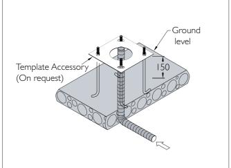
Height of foundation above ground level (150mm) may be revised to suit the site conditions especially considering the expected water level stagnation during heavy downpour.
