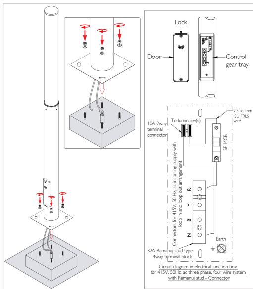
Please ensure that the wires are connected to the right polarity [Phase, Neutral & Earth]. For 3Phase Loopin Loopout connections, use appropriate Red, Yellow, Blue for Phase, Black for Neutral and Green for Earthing Terminals.
