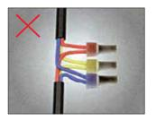
When the wire is connected into the fixture through cable gland, the cable must be more than 10mm inside. Please refer to the images below.
