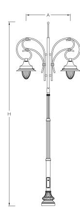
**Finish:** Coated with epoxy zinc phosphate primer and finished using environmentally stable polyurethane based paint.
