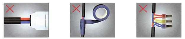
When the wire is connected into the fixture through cable gland, the cable must be more than 10mm inside. Please refer to the images below.
