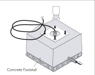
Template (On request) supplied is suggested to be used for locating the centre to centre (CC) distance of foundations bolts
